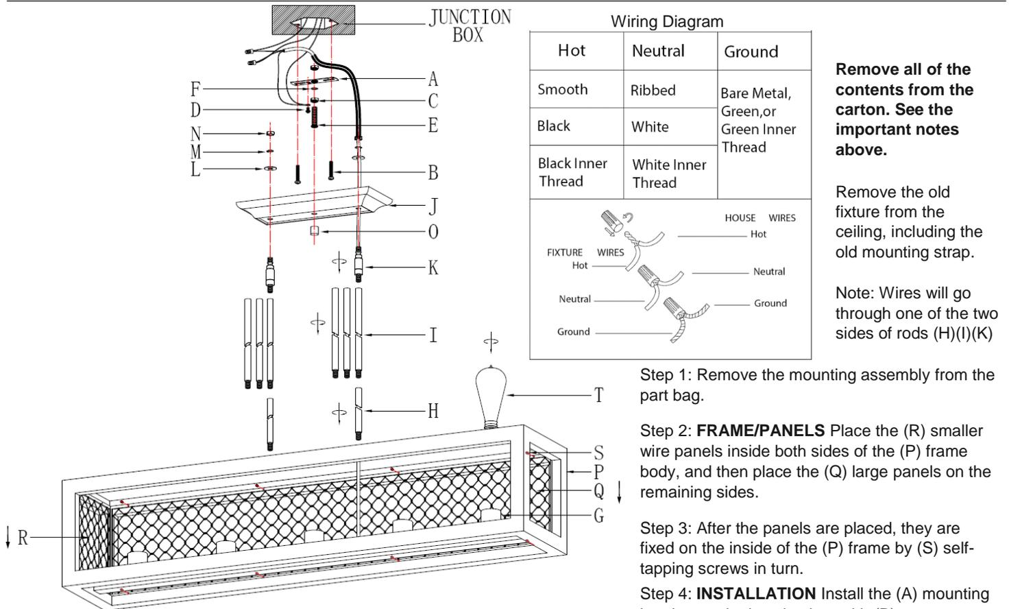
Step 5: Install the (F) washer, (C) nut, and (E) tooth segment on the (A) mounting bracket in turn.
