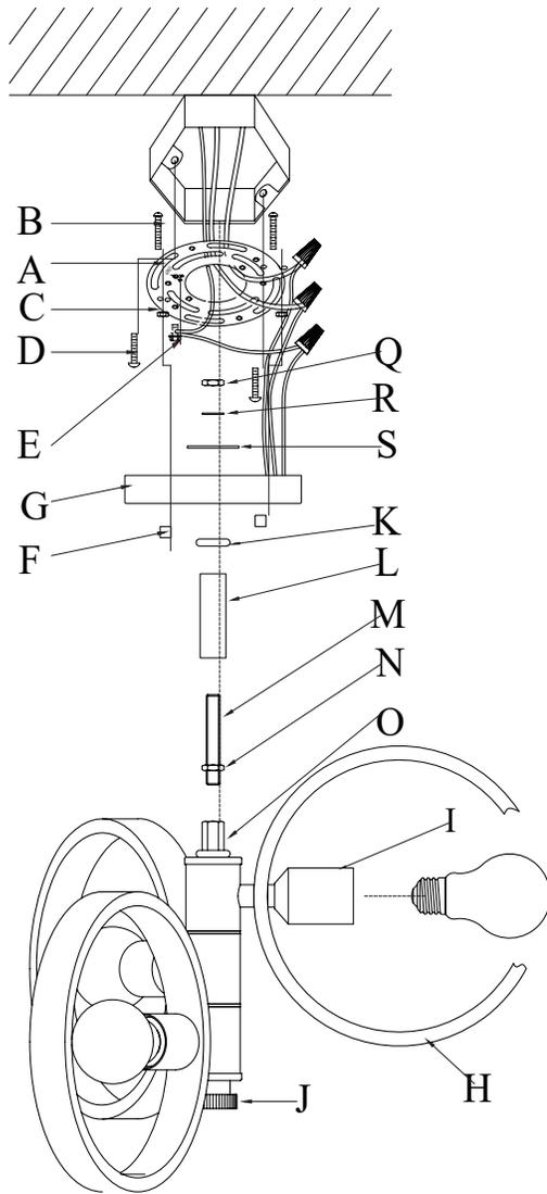
**Important Note:** To avoid snapping the fixture's wires, do not fully twist rings (H) more than 2 times in the same direction. Instead twist the rings in the opposite direction to achieve the look you desire.
